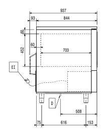
Drain Electrical inlet (power)
